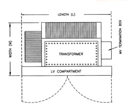
FIGURE-1: UNIT SUBSTATION COMPONENT LAY-OUT
