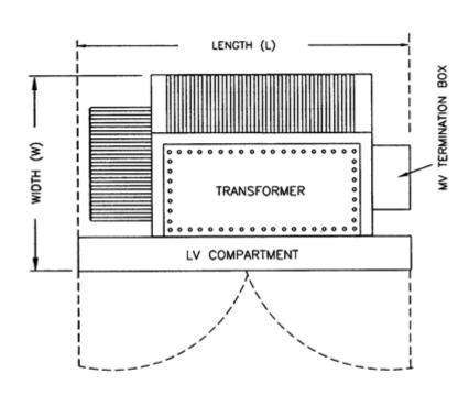
FIGURE-1: UNIT SUBSTATION COMPONENT LAY-OUT
