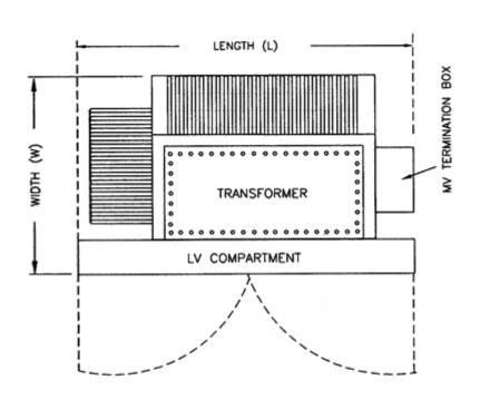
FIGURE-1: UNIT SUBSTATION COMPONENT LAY-OUT
