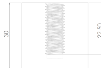
Drawing No. 13.0: Details of Stainless-Steel Threaded Blind Nodes for Fixing the Wall-Mounting Brackets at the Back of the Meterboxes
