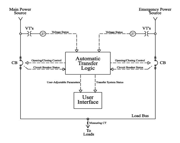
Figure 2: Typical LV ATS Key Diagram
