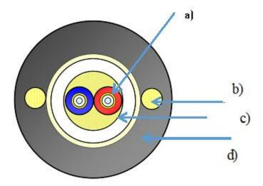
**Legend:** a) 900 Microns Colored buffered fiber, b) Glass Reinforced Plastic Longitudinal strength Member c) Dielectric Strength Reinforcement Member d) White or Ivory LSZH Outer sheath
